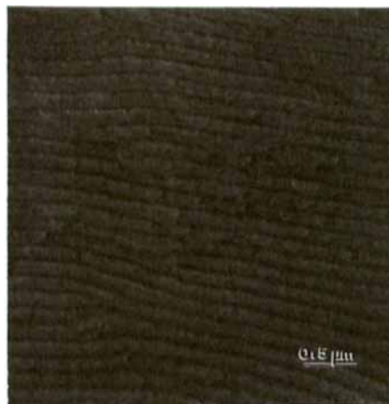
Figure 7. LVHRSEM (0.8 keV) micrograph of bulk fracture surface from the sample investigated.
